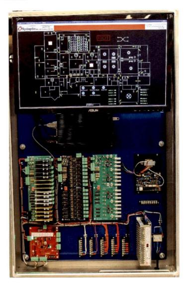
The security control cards are on the left on a green motherboard, middle is an intercom security control board which is black, and on the right is a video selector board which is green, intercom amp is far right and is black. Bottom left is the Node board which acts much like a PLC and is red. Power supply is lower right. Directly below the screen showing a fictitious floorplan is the fanless PC. All of our wiring is color-coded as well.
