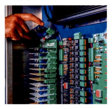
As an example of our 1220 control system. Pictured below is our training unit. This unit goes to the facility and while the old system is being removed and the new Sydaptic system is being installed, programmed, and tested, this system is used to train the staff on the new system's operation.
